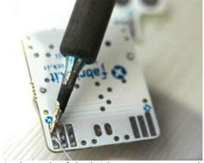
tin the pads of the brick you want to attach the ribbon to
