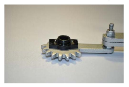
There is a technique to this. Push the plastic servo horn against the robotic claw gear and screw the screw through the servo horn. If you do not apply pressure, the screw will just simply push the servo horn out. Be careful while doing this, the screw might poke your finger.
