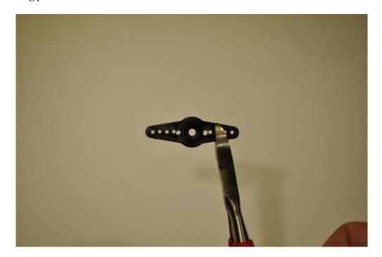
Cut it precisely at the edge of the 3<sup>rd</sup> hole closest to the center of the horn. This ensures that the horn does not bump into other parts of the claw and allows the servo to rotate freely, which also allows the claw to open and close properly.
