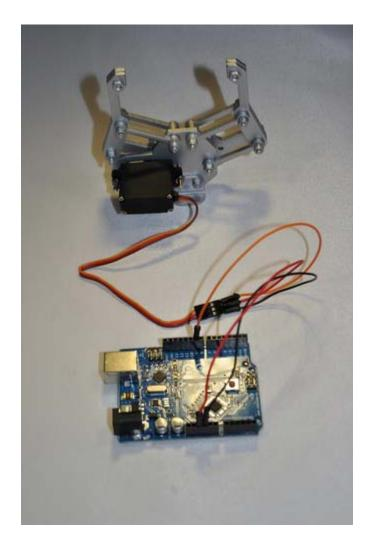
One of the quickest ways to see if your claw is working is to hook it up to an Arduino. I used an Uno, but any 5V Arduino compatible board can be used to control the claw.
