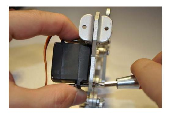
This picture was taken at an angle behind the robotic claw. At the top, you can see the robotic claw's mounting plates. To the right of the servo, protruding from the other side of the robotic claw, you can see the golden servo gear. You want that gear to be parallel with the robotic claw.
