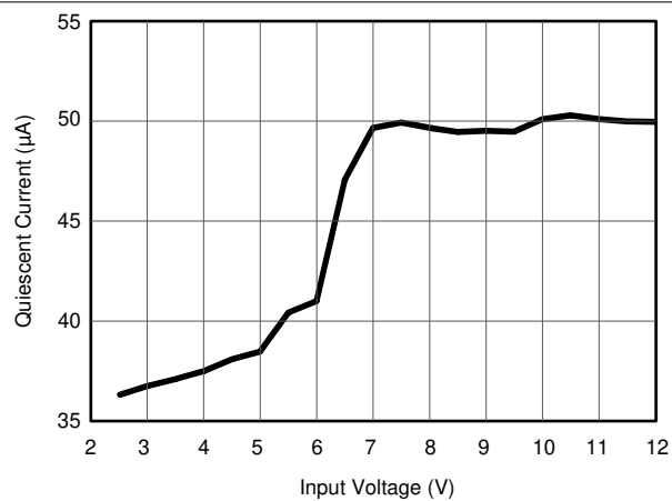
Figure 7-2. Quiescent Current vs Input Voltage
