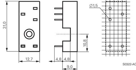
**RP 78 602** Socket with PCB terminals, pinning 5 mm
