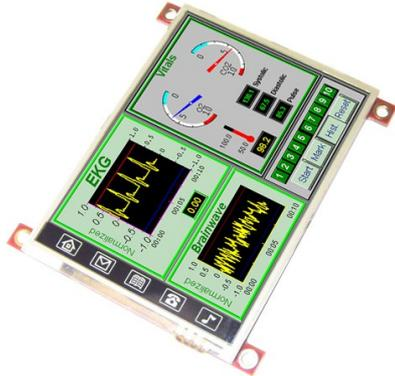
The **μLCD-32PT(SGC)** is a compact and cost effective all in one ‘SMART’ serial display modules using the latest state of the art LCD (TFT) technology with an embedded PICASO-SGC serial graphics controller that delivers ‘stand-alone’ functionality to any project.
