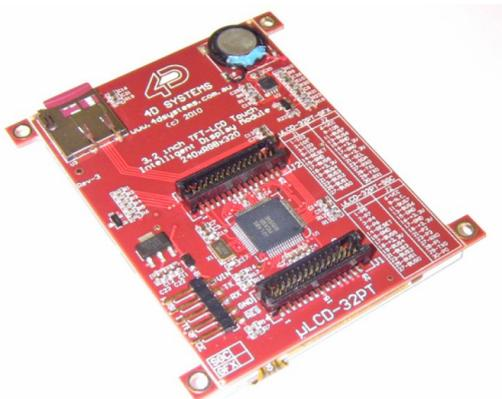
The serial platform allows users to develop their application using their favourite micro-controller and software development tools. In short, the μLCD-32PT(SGC) display module offers some of the most flexible embedded graphics solutions available.
