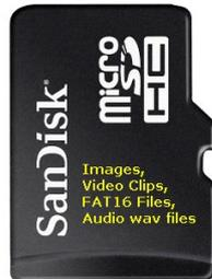
The module also support high capacity HC memory cards (4Gb and above). The available capacity of SD-HC cards varies according to the way the card is partitioned and the commands used to access it.
