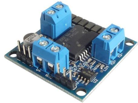
The *DC Dual Motor Driver 30V 4A V2* allows to independently drive two DC motors, controlling both velocity and direction.
