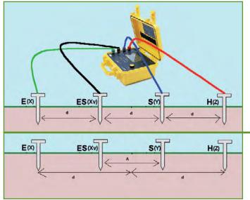
Wenner method: the distances between the 4 rods are identical: (d) pW=2. ?.d.RS-SE
