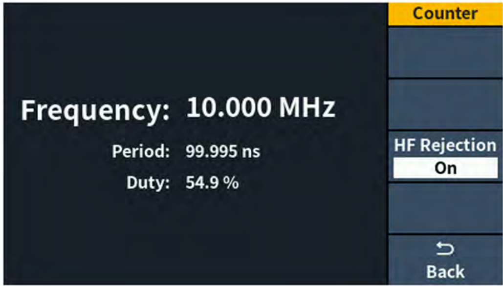
Frequency counter function: High-accuracy frequency counter integrated, supported range 100mHz - 100MHz
