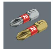
BTH- (extra-hard) and BTZ- (tough) bits have an additional tempered BiTorsion zone, which reduces the hardness of the shaft by about 20 % in comparison to the drive tip. This means that the peak loads that cause bit breakage and premature wear are absorbed in this zone — something which enhances the service life of the bits.
