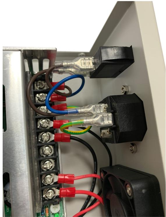
7. Connect the black cable of the fan control to the power supply with one of the anticipated terminals V- and the red cable with one of the V+ terminals.
