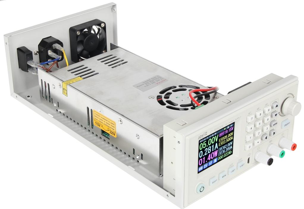
You can adjust with the help of the fine-tuning potentiometer the output voltage of the RD6006-NT. You can see your adjustment at the input voltage of your RD6006. Ideally, the RD6006 has a input voltage of 65 V to be able to issue the complete 60 V.
