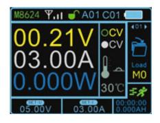
If the load current is below the set current, the output is a constant voltage. The CV light comes on.
