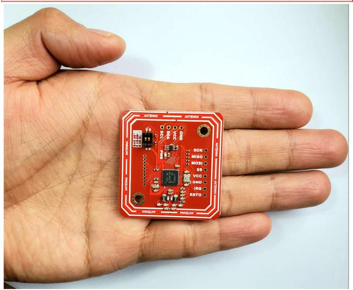
**Near field communication (NFC)** is a set of standards for smartphones and similar devices to establish radio communication with each other by touching them together or bringing them into close proximity, usually no more than a few centimeters.
