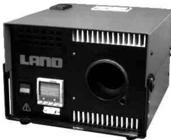
Fig. 1 Landcal Blackbody Source Type P80P
