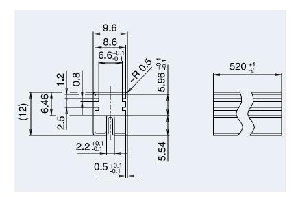
Tube for THT version 50 relays per tube 1'000 relays per box
