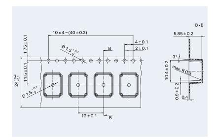
Tape and reel for SMT version 1'000 relays per reel 1'000 or 5'000 relays per box
