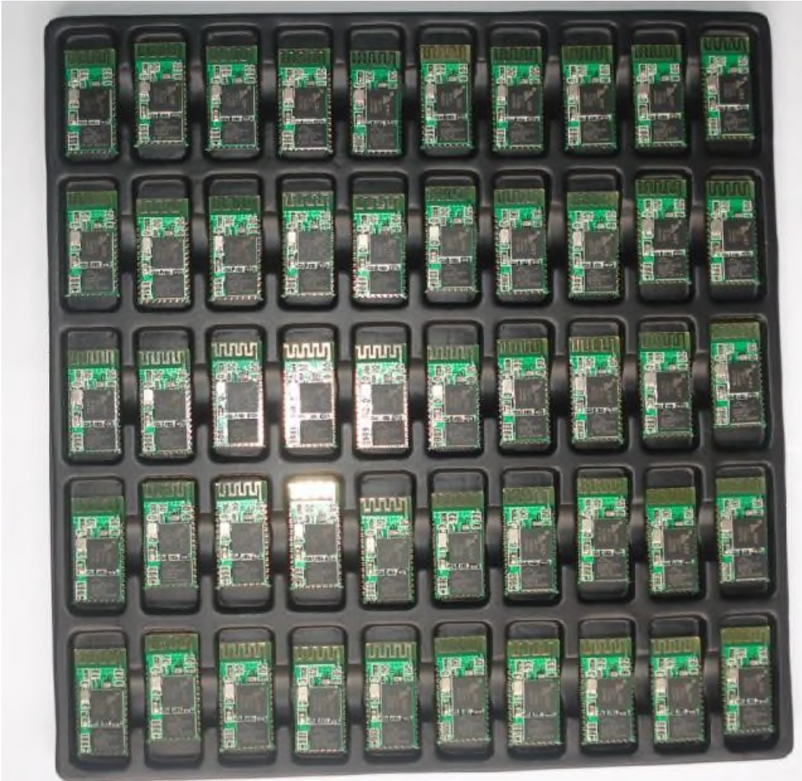
Figure 2 50 pieces chips in an anti-static blister package
