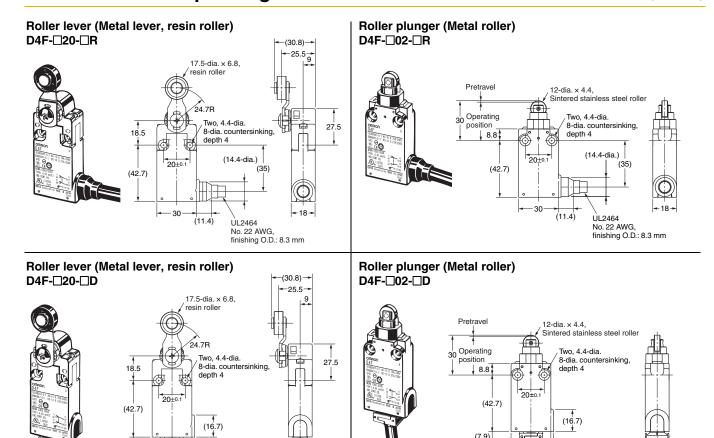
Note: Each dimension has a tolerance of 0.4 mm unless otherwise specified.
